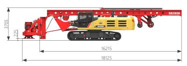
High-efficiency in rock drilling: The medium-sized Sany rotary drilling rig with the largest sales volume, equipped with the newly upgraded sixth-generation Kelly bar of integral locking device, upgraded materials, and reinforced rings, etc., to make rock layers construction capacity improved by 10%.
